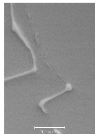
Figure 5 – Fine, discrete grain boundary carbides in CM 939 Weldable after heat treatment
