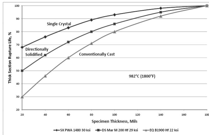
Figure 2. Rupture life vs. specimen thickness showing benefit of SX castings over DS/EQ
