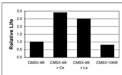
Figure 13 – Reactive element effects on EB-PVD TBC life
