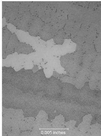
Figure 4 – Microstructure of CM 939 Weldable following heat treatment
