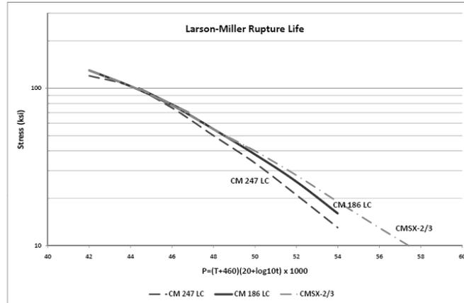
Figure 9 – Larson-Miller stress rupture life of DS CM 186 LC, DS CM 247 LC and SX CMSX-2/3
