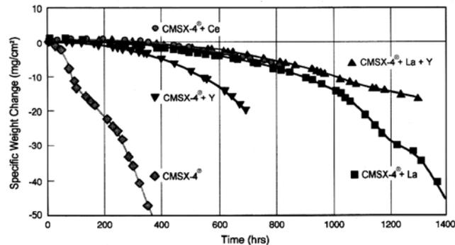
Figure 11 – 1093°C (2000°F) dynamic cyclic oxidation results for bare CMSX-4 alloy with and without reactive element additions
