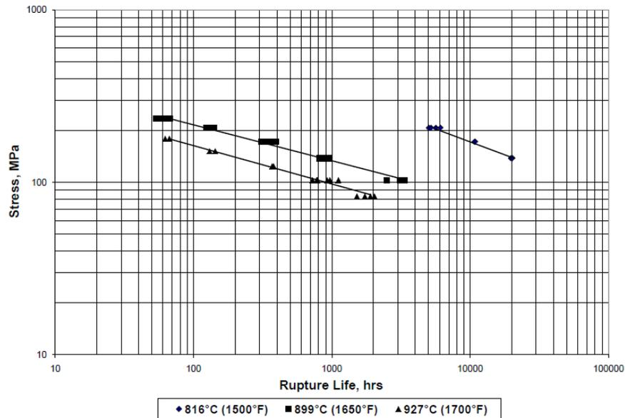
Figure 6 – CM 939 Weldable stress-rupture life (five step thermal treatment)
