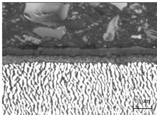
Figure 12 – Surface microstructure on CMSX-4 [39 ppm La+Y] following creep-rupture testing at 1050°C/125 MPa (courtesy Rolls-Royce plc)
