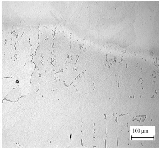
Figure 7 – Typical weld microstructure at the CM 939 Weldable/C263 filler metal fusion line
